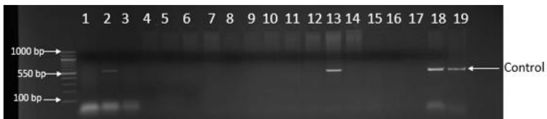
Plate 5. Electrophoresis of PCR products for bla CTX-M . Lane 2 – E. aerogenes from an ewe, Lane 13 – E. coli from a doe, Lane 18 – K. oxytoca from a cow, Lane 19 – Control.
