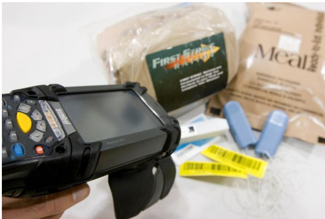
Figure 4. Portable barcode scanner (Credit: Tyler Jones, UF/IFAS).
