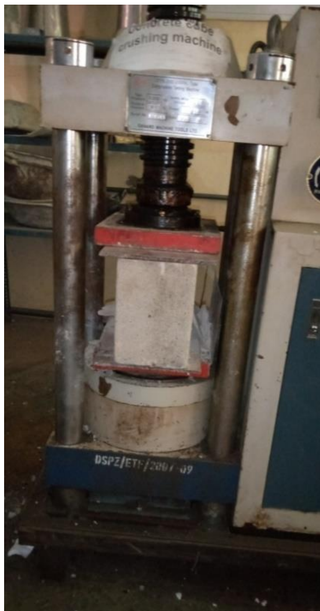
Figure 3. Sandcrete block undergoing compressive testing.
