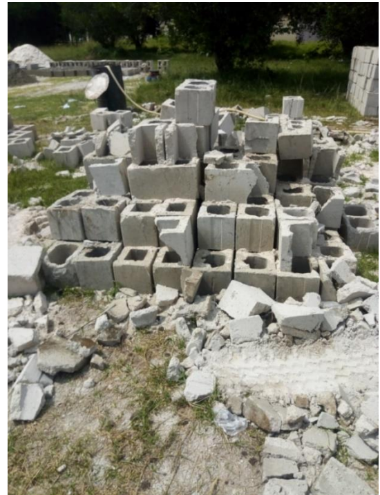
Figure 11. Broken sandcrete blocks littering a construction site in Delta State, Nigeria.
