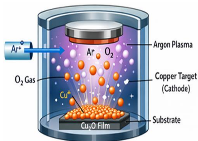
Figure 4. Schematic illustration of the reactive magnetron sputtering system used for \text{Cu}_2\text{O} thin-film deposition, showing the copper target, plasma region, and substrate (Aghilzadeh et al. , 2017).
