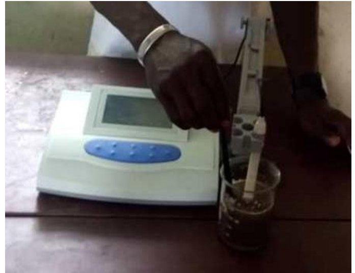
Figure 2. Determining the electrical conductivity of soil samples.
