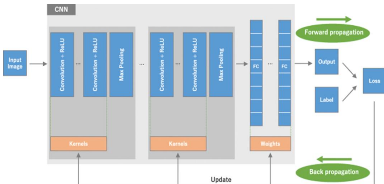
Figure 1. Convolutional neural network (CNN) architecture and the training process (Source: https://insightsimaging.springeropen.com/articles/10.1007/s13244-018-0639-9/figures/1 ).
